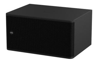
The Venu 215 V2 is a double 15" reflex-loaded low frequency enclosure, providing a frequency response of 38 Hz - 160 kHz  $\pm$ 3 dB and efficiency of 99 dB. Features include tough 15" high excursion transducers with 4" voice coils and a durable enclosure made entirely from 18 mm multi-laminate birch plywood.
